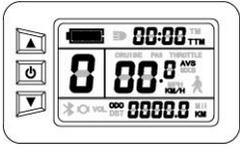
Hold ⏻ button shortly in display 1 to enter display 2. In the riding mode after 5 seconds, display 2 automatically returns to display 1.
